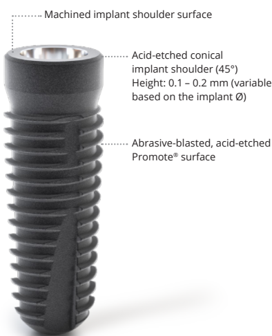
CONELOG® SCREW-LINE Implant Promote® plus
