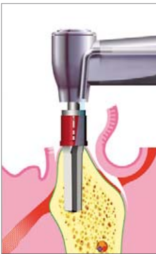
Example: Form drilling Ø 4.3 mm
